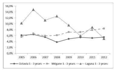
Figure 1. Percentage of cars with serious defect. Source: own on the base of TÜV data.
